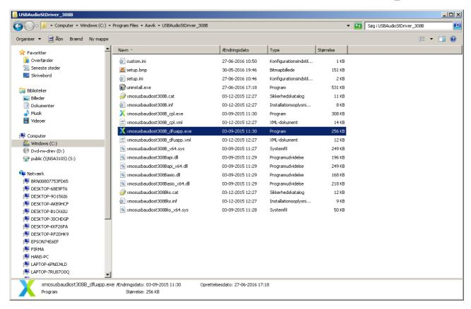
Run the firmware update tool (xmosusbaudiost308B\_dfuapp.exe). The DAC/amplifier has to be switched on, and you should see the "Device opened." text.
