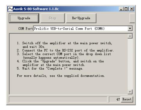
The "COM Port" dropdown list usually select the correct serial port automatically. You can find a list of serial ports in your PC by using "device manager"
